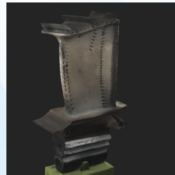
Figure 2. (a) Use of photogrammetry to reconstruct a CAD model of the HPT turbine from 72 images, which are taken at 15° intervals from three different locations. (b) The resulting CAD model.
