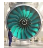
TC3: Ultra High Bypass Ratio fan
